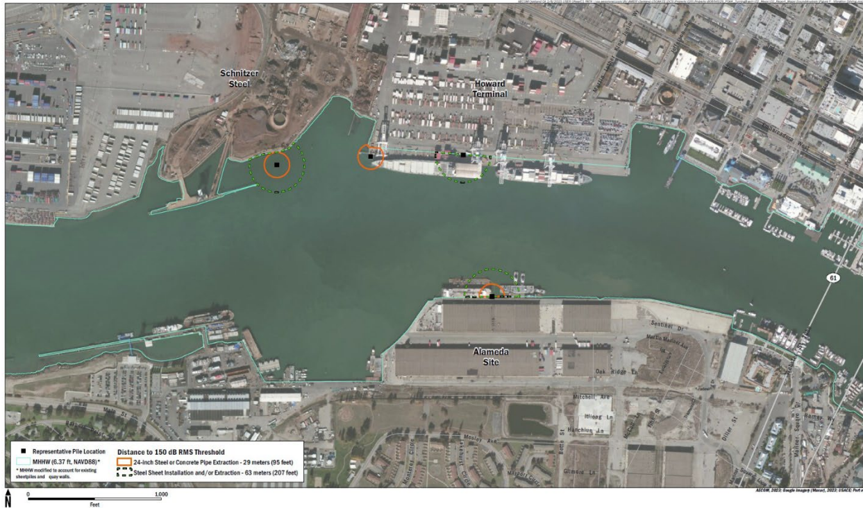
Figure 6-6 Estimated Distance to In-Water Sound Pressure Criteria for Fish for Vibratory Driving
